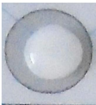
I hope you obtained something like this. The white precipitate of barium sulfate suddenly appears. The technique makes use of the hydrophobic properties of the plastic. (I prefer polypropylene.) My thoughts went to carrying out many more precipitation reactions similar in the same manner and establishing solubility rules. See the sheet I drew up. I put in some mixtures not giving a precipitate as well.
